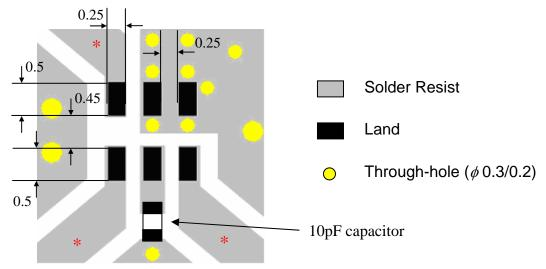
• Line width should be designed to match  $50\Omega$  characteristic impedance, depending on PCB material and thickness.
